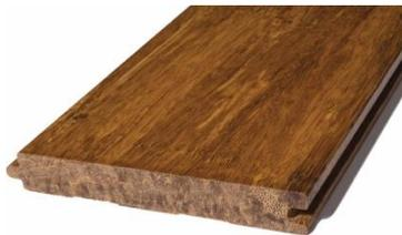
The second category is Strand Woven bamboo. In this second-generation bamboo construction, thousands of sawn bamboo strips are partially shredded to open up and expose bamboo's highly resilient stringy fiber. Resins are added to these strips, which are then pressed together under tremendous pressure. This produces a densified bamboo and resin composite product that is harder and far more durable than Traditional bamboo flooring.
